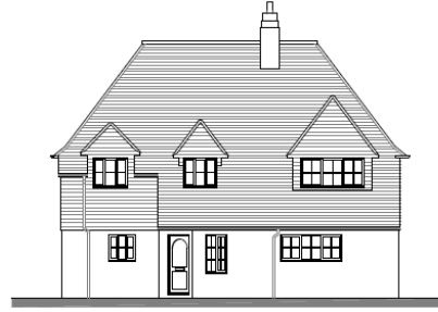
EXISTING NORTH FACING ELEVATION Sc. 1:100
